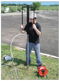
Installing Piezometers with a Manual Slide Hammer
