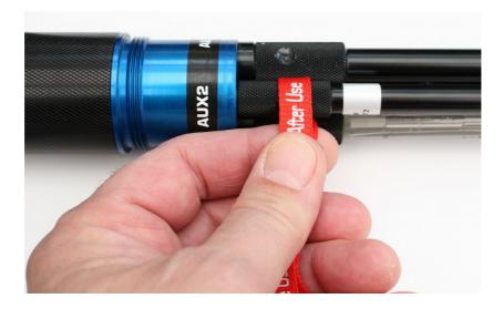
Apply a small amount of silicone grease (supplied with the Aquaprobe®) to the threaded section and the O-ring of the AUX Electrode (see photograph). **ENSURE NO GREASE IS APPLIED TO THE GOLD CONTACTS**.
