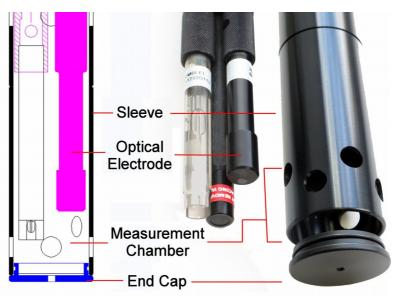
In order to obtain consistent results, the measurement chamber created within the Aquaprobe® must remain physically constant during both calibration and measurement.
