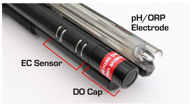
Please note: The photograph shows the AP-2000 with Optical DO. The AP-700 and AP-800 models may have either Optical DO or Galvanic DO sensors.
