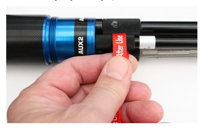
Slide the lanyard over the electrode and use it to grip the knurled body.
