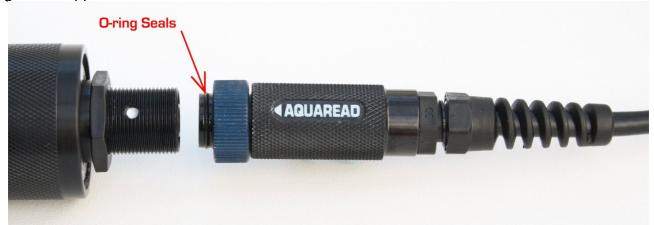
Apply a generous smear of grease to the O-rings where indicated above. Be careful not to get any grease inside the connector near the gold contacts. A small smear of grease should also be applied to the thread on the Probe to allow easy tightening of the collar.
