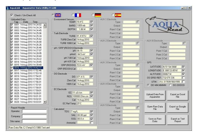
To view any of the logged data records, simply click on the desired Tag, date and time label as shown above. The data for the highlighted label will be displayed in the individual data boxes, which are grouped by electrode function. Any data that is unavailable or out of range will be displayed as dashes. To move up and down the Tag/date/time column, use either your mouse or the cursor up/down keys.
